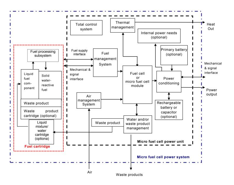
Figure 1.1 – Micro fuel cell power system block diagram for UN Division 4.3 (water reactive) compound fuel in indirect PEM fuel cell system – Fuel management system in micro fuel cell power unit
